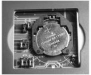
This battery socket accepts a 3 V button cell Lithium battery (CR2032) required to support the system real time clock. The jumpers in this window are designated for COM port power supply function. Please consult your dealer for technical support on setup of these jumpers. A new Lithium battery can support the system RTC for about 3 years. After the battery is nearly exhausted, the user must change a new battery otherwise the system RTC and system configuration setup will be lost.
